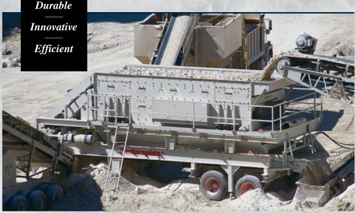
Cedarapids/ElJay Legacy Series Screens provide the contractor with proven performance. The ability to change stroke angle, amplitude and speed to meet changing screening conditions makes this versatile screen highly efficient in most any application. Smooth operation, virtually non-plugging, exceptional bearing life and simplified adjustment procedure make the Legacy ideal for either stationary or portable applications.
